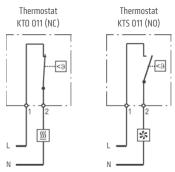
Filter fan, Cooling equipment, Signal device
